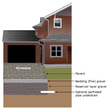
Existing soils that allow infiltration at  ${\bf 1}$  inch per hour minimum if soils do not have a lot of clay, preferably  ${\bf 2}$  inches per hour.
