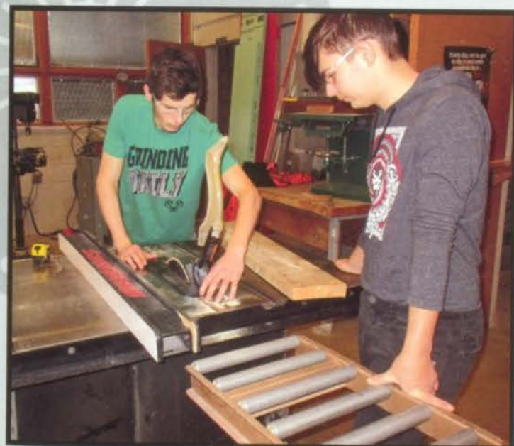
G. Ingram and L. Miller are making adjustments to the depth of the blade on this table saw. It's important that it cuts through the wood without having a large amount of the blade exposed.
