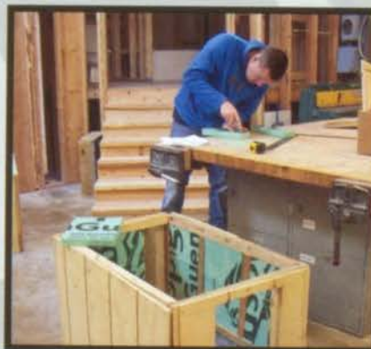
M. Burge measuring and cutting pieces of Styrofoam insulation which will help keep the inside of the dog house warm and free from drafts.
