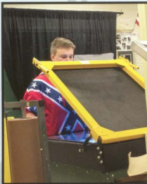
E. Powell sets up his screen to be exposed to light. This process is the one of the first steps to create a silk screen print.
