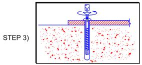
TO REMOVE: PRESS A No. 2 SCREWDRIVER FIRMLY INTO THE SCREW HEAD AND TURN COUNTER CLOCKWISE. PRY THE SCREW FROM THE ANCHOR BODY, THEN PRY OUT THE FIXTURE AND ANCHOR BODY.
