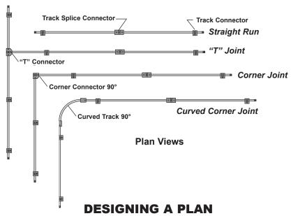
The design of your curtain assembly will be determined by the position of roof trusses or beams and any obstructions such as shelving or structural columns. Clearly mark where each Beam Clamp, either Splice or Track Connector, will be attached to the trusses since the track assembly will fabricated "on the ground" before it is secured to the roof trusses.
