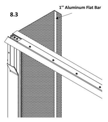
At this point the side screens might need to be trimmed using scissors or a utility knife. The screen should be 3" wider than the distance from the guide track to the wall. Carefully place the excess material against the wall, fold material toward the doorway opening and use appropriate fasteners (not included) to pinch the side screen between the flat bar and the wall. (8.3).
