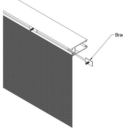
Slide the bracket anchor plates into the guide channel that is on the outside edge of the track guides. Evenly split the bracket anchor plates between the guide tracks.
