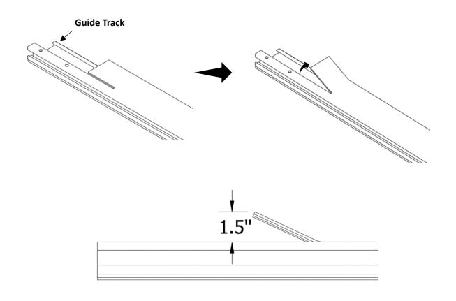
Slide each side screen into the groove that is at the bottom outside edge of the track grooves.
