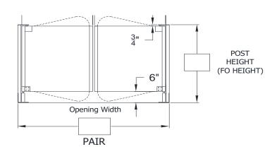
**STANDARD SPECIFICATIONS**: Door body 0.063" tempered aluminum alloy, satin anodized finish. No contour is standard. Door assembly includes the original Easy Swing® hinges installed on black powder coated freestanding gate post. (FO Height Minimum 24", For Maximum see table: Post Height Maximum 54")
