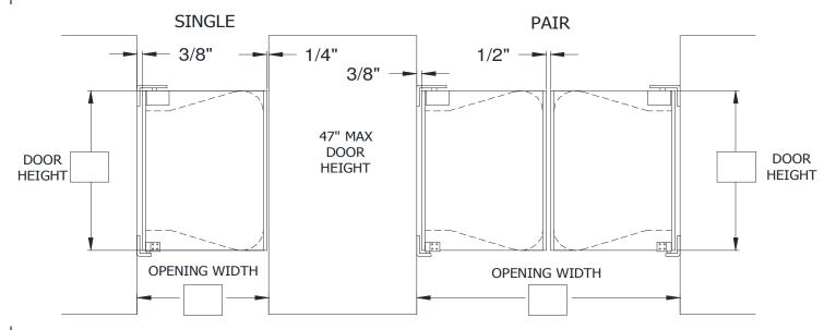
**STANDARD SPECIFICATIONS:** Door body .063" tempered aluminum alloy, satin anodized finish. Door assembly includes the original "NO SPRING" Easy Swing® hinges and both 1/4" - 20 x 1" thread cutting screws and #14 -1-1/2" sheet metal/wood screws for jamb by others. (Minimum cafe/gate height is 24")
