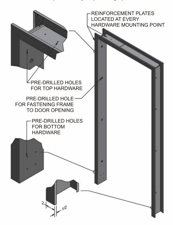
ROUGH OPENING WIDTH = FINISHED OPENING WIDTH + 4 1/2" ROUGH OPENING HEIGHT = FINISHED OPENING HEIGHT + 2 1/4"
