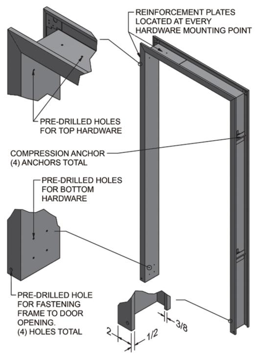
ROUGH OPENING WIDTH = FINISHED OPENING WIDTH + 2 3/4" ROUGH OPENING HEIGHT = FINISHED OPENING HEIGHT + 1"
