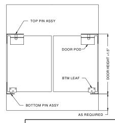
JAMB MUST BE SQUARE AND PLUMB A MINIMUM OF 3-1/2 INCH WIDE JAMBS REQUIRED TO MOUNT HARDWARE
